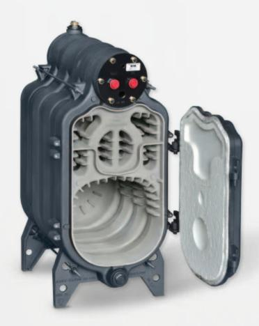
The new Saint Roch COMBI Boiler is a high efficiency, triple pass, multi-fuel boiler equipped with a cylindrical coil chamber on top. The coil chamber can be used to produce DHW using Hypoeutectic, Grey Cast iron, Saint Roch COMBI boilers are cast for strength and durability, The heat exchanger is designed with multiple finned columns which direct boiler water flow to scrub the finned coil in the chamber above the heat exchanger.
